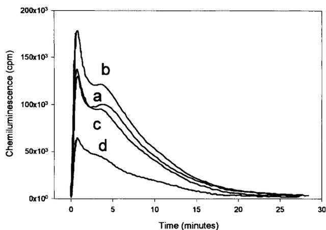
**Fig. 4.** CL produced by milled anthophyllite samples.
