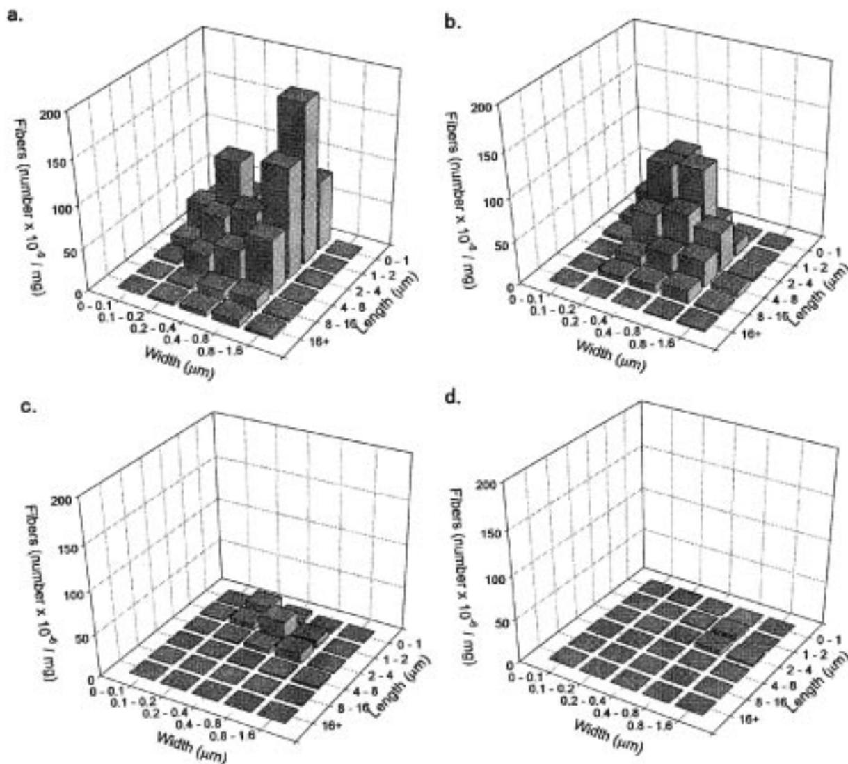
**Fig. 1.** Changes in the size distribution of glass fiber samples with duration of the milling.
