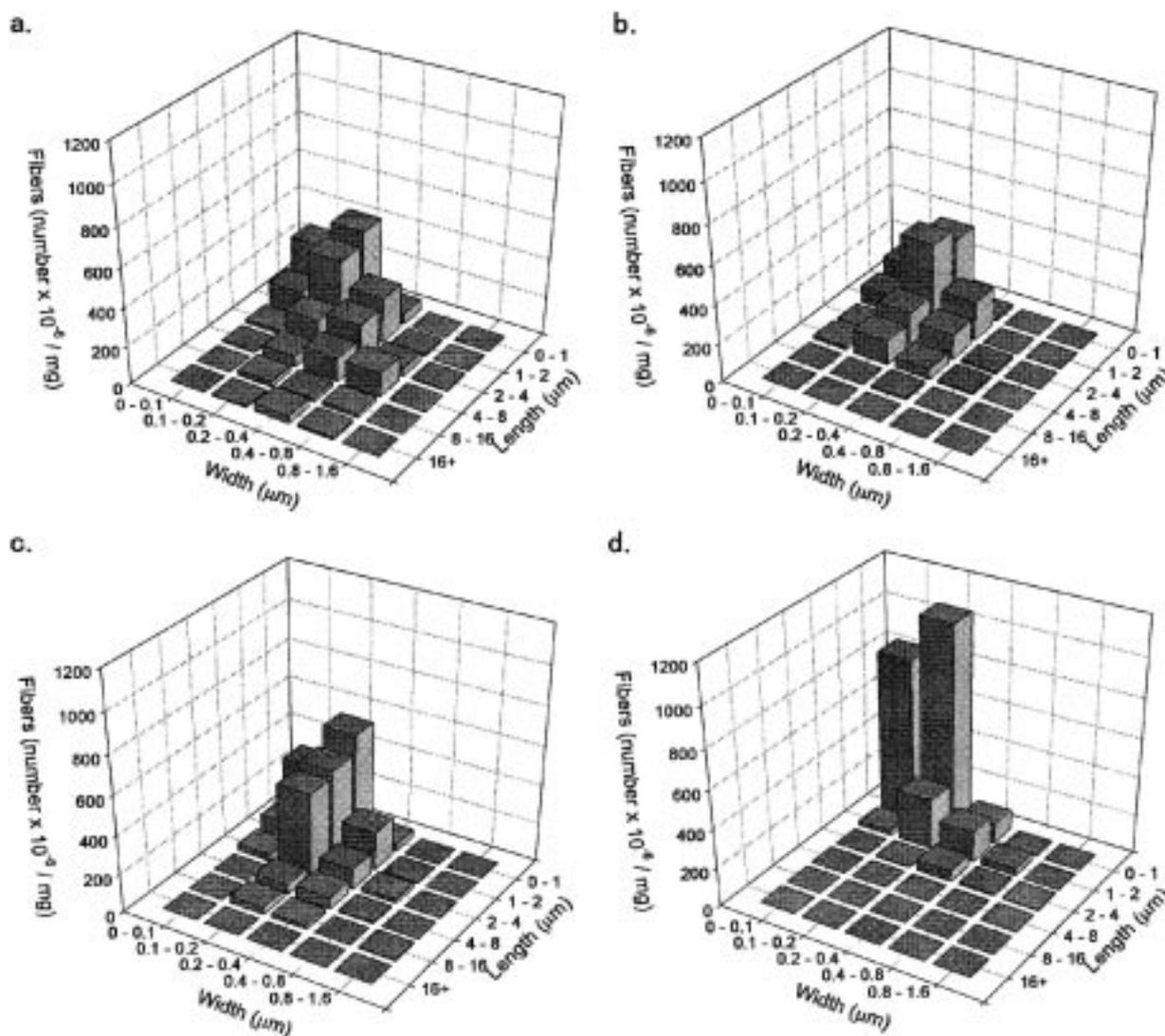
**Fig. 2. Changes in the size distribution of anthophyllite samples with duration of the milling.**
